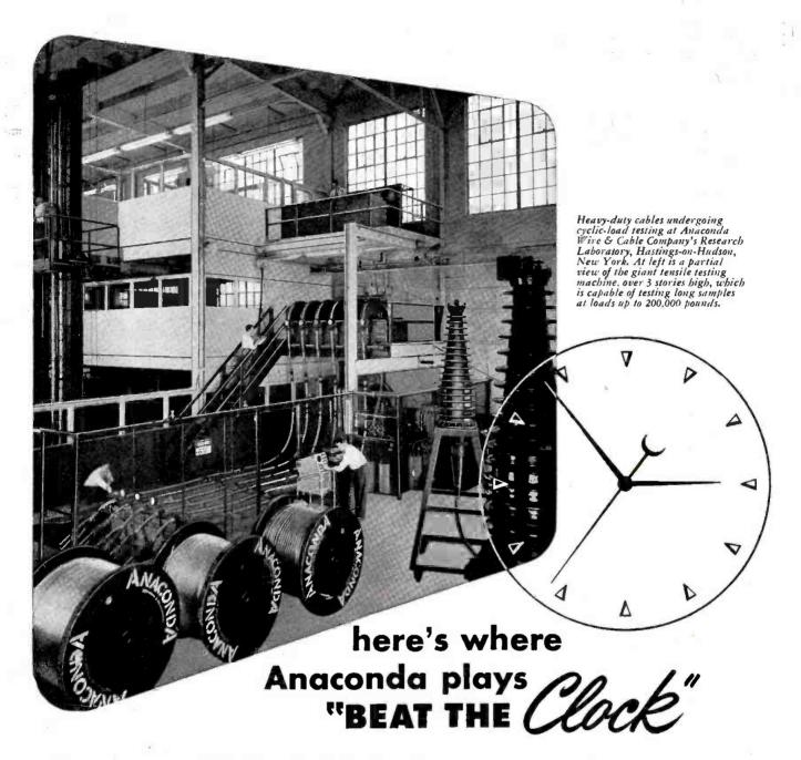
Years are compressed into minutes in the Cyclic Aging Laboratory of Anaconda's subsidiary, Anaconda Wire & Cable Company, at Hastingson-Hudson, N. Y. Here, through rigorous 24-hour testing cycles simulating actual conditions but decidedly more severe, high-voltage insulated cable is tested for long life, stability, and other desirable characteristics.
