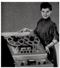
AMPEX Model 350, new tape recorder developed by Ampex Electric Corp., features 30-degree slope on both tape transport and control sections. Machine is designed for easy servicing.
