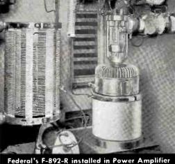
Federal's F-892-R installed in Power Amplifier Section of WMCA's 5000-watt Transmitter
