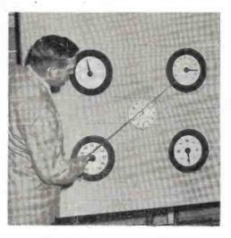
est wind velocity instruments, including an Aerovane, made by Bendix-Frieze, are installed on the WBAP-TV roof, from which readings are transmitted to the studio instruments by selsyn-synchronous motors. The temperature is transmitted the same way, over underground cables connected to a permanent weather house adjacent to the building.
