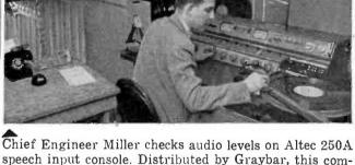
Chief Engineer Miller checks audio levels on Altec 250A speech input console. Distributed by Graybar, this completely self-contained unit provides all necessary monitoring, cue, audition, and signaling circuits for WNAO's audio control.
