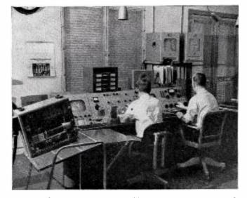
Two engineers control WNAO's entire program schedu slides, film, studio and network – with Federal Transm Control Console and Poly-Efex Scanner providing com transmitter supervisory control and audio/video switch Scanner includes 2 slide sources, four-channel video swit and "special effects" section.
