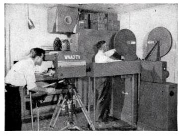
Engineers W. F. Anderson and L. E. Rudisill set up the late evening film show on WNAO's General Precision Laboratories 16mm projectors. The FTL image orthicon camera is also used for interviews and newscasts originating "live" in a small studio here at the transmitter building.
