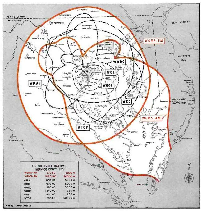
WGMS-AM five kilowatts day, one kilowatt night; contours computed for WGMS, measured for others.
