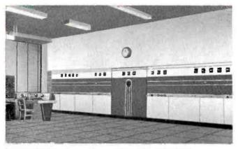
RCA 50-KW Shortwave Transmitter using RCA-857B high-power mercury-vapor rectifiers
