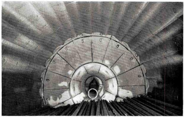
For A Tough Grind. This mill is used to grind the highly abrasive, low-grade iron ore called Taconite. Rolled Steel Plate Lining, bolted to the inside surface of the large revolving cylinder, lifts and tumbles the load and also protects the shell from the grinding action of the steel rods and the ore. This lining, especially made for such service, processed 1,100,000 tons of Taconite—another outstanding performance of USS Lorain-Rolled Plate Linings.
