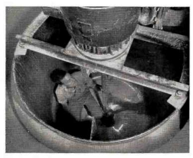
The Finest Printing is Done on Clay. High-gloss papers (called enamel-coated) are covered with a thin coating of smooth, hard, lustrous clay to keep printing inks from being absorbed into the paper fibers. That clay is mixed in tanks like this one. Tanks are stainless steel because nothing else can withstand the grinding action of the clay and at the same time keep it pure and white. In fact, this stainless tank has lasted seven times as long as the previous non-stainless tank.
