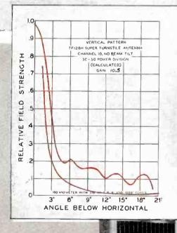
Vertical Field Pattern of new RCA TF-12BH 50-kw antenna. Note complete absence of vertical nulls. Operated in conjunction with an RCA 50-kw TT-50AH transmitter, this antenna will "saturate" your service area with strong signals.
