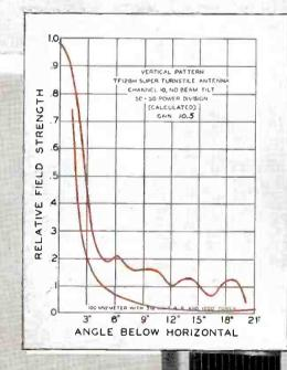
Vertical Field Pattern of new RCA TF-12BM 50-kw antenna. Note complete absence of vertical nulls. Operated in conjunction with an RCA 50-kw TT-50AH transmitter, this antenna will "saturate" your service area with strong signals.
