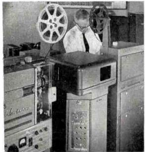
**PROTECTION SYSTEM.** RCA TP-6 16 mm professional projectors are used to double-up with 35 mm network projectors to insure on-air continuity in event of mishap. TP-6's are used throughout ABC local film rooms.
