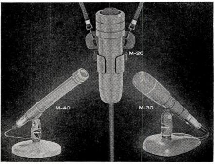
M-40 response 40-20,000 cps • output -57 db • 9½ inches long, I inch in diameter • II ounces. M-30 response 50-18,000 cps. • output —57 db • 6½ inches long, 1¾ inches in diameter at head • 16 ounces. M-20 response 60-18,000 cps. • output —57 db • 4 inches long, I inch in diameter . 31/2 ounces. For more information contact your Collins sales engineer or write.
