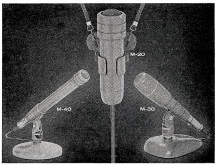
M-40 response 40-20,000 cps · output -57 db · 9½ inches long, 1 inch in diameter · 11 ounces. M-30 response 50-18,000 cps. • output -57 db • 6½ inches long, 1¾ inches in diameter at head • 16 ounces. M-20 response 60-18,000 cps • output -57 db • 4 inches long, 1 inch in diameter • 31/2 ounces. For more information contact your Collins sales engineer or write.
