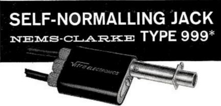
This self-normalling jack is for use in applications where a "normalthrough" condition is known to be of a semi-permanent nature. It accepts a Nems-Clarke 966-A or 967 series patch cord plug for sampling or temporary re-routing. So used, the rear jack connection is automatically terminated to 70 or 50 ohm impedance. Removal of
