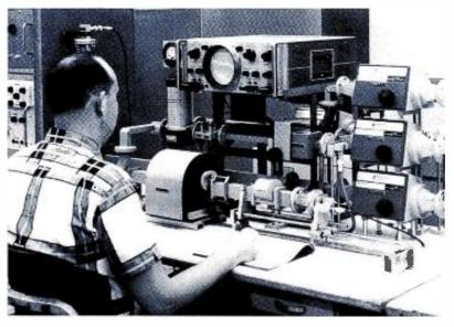
In defense electronics... broad-band microwave attenuators built by H-I's PRD Electronics division serve in production-line testing at Western Electric Company, Allentown, Pa. Here a series of PRD attenuators is used to adjust and test ferrite isolators. PRD manufactures microwave instruments and electronic measurement systems for government agencies and defense contractors.
