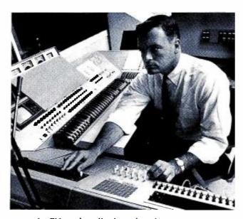
In TV and radio broadcasting...new multimillion-dollar CBS Broadcast Center in New York utilizes seven Gates custombuilt, solid-state consoles like this for finger-tip control of all audio. Transistorization is carried to a point never before realized in a broadcast facility of this size.
