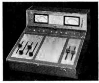
as low- or medium-level inputs—a selector switch chooses. Two mixer buses, two program/monitor amplifiers, built-in cue facility, one VU meter with provision for adding second.
