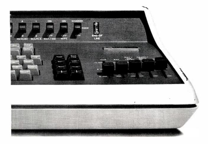
sponsibility. Built into the TCG-1425A is a solid-state switcher which permits selection between two video sources. The source selected is routed through the matting amplifier while the other source is bypassed through an equivalent delay circuit. One of the sources even has a fail-safe metallic-contact bypass.
