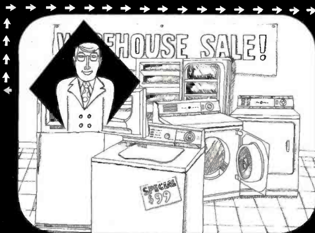
3 Non-repeat feature allows a pattern to be positioned completely off screen without reappearing on opposite side of picture. This feature also allows male announcer to be "walked" off screen in a diamond pattern.
