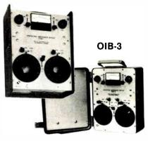
The Operating Impedance Bridge measures the impedance of networks, radiators, and the like while they operate under full power. VSWR as well as complex impedances of up to 400  $\pm$  j300 ohms can be measured.
