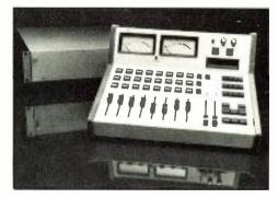
input ESAM system provides edit system control of source selection, preview functions and transitions and is configured to operate like a video switcher. The \$8,750 unit can also be operated manually as a conventional audio mixer. Delivery is scheduled to begin this month.
