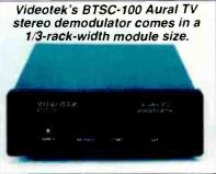
or composite aural input into both stereo and SAP (second audio program) baseband audio outputs. The unit is designed for cable TV applications, and can be used in headends or other distribution locations where aural information is available and wherever there is a need for local baseband audio insertions. In addition to providing high-guality stereo and SAP outputs, the BTSC-100 also provides a composite aural output from a 4.5 mhz IF input.
