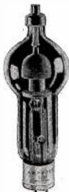
*Amperex* Type 575-A Mercury Vapor Rectifier. Filament AC voltage, 5.0 volts. Filament current, 10.0 amperes. Preheating period, before plate voltage is applied, 30 seconds. \$30.00, list price.
