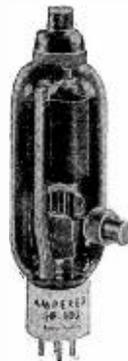
*Amperex* Type HF-100 Transmitting Tube. Filament Voltage, 10-10.5 volts. Filament current, 2.5 amperes. Amplification factor, 23. Grid to plate transconductance at 100 ma., 4200. Direct interelectrode capacitance: Grid to plate, 4.5  $\mu\text{f}$ ; grid to filament, 3.5  $\mu\text{f}$ ; plate to filament, 1.4  $\mu\text{f}$ . \$12.50, list price.
