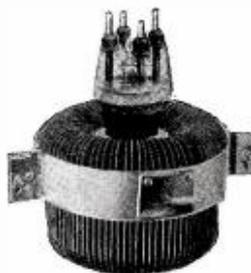
*Amperex* Type 889-R Transmitting Tube. Filament voltage, 11 volts. Filament current, 125 amperes. Amplification factor, 21. Direct interelectrode capacitance: Grid to plate, 20.7  $\mu\text{f}$ ; Grid to filament, 19.5  $\mu\text{f}$ ; Plate to filament, 2.5  $\mu\text{f}$ . \$260.00, list price.
