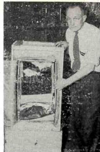
**MORE "GARMENTS"** than most people would want in a tropical wardrobe "clothe" the RCA Victor electronic equipment in this outaway view of a moisture-proof package prepared for shipment to the tropics. This kind of packaging, coupled with tropicalization treatment of equipment and parts, can give longer life to radio and electronic equipment by protecting it against damage from fungus, corrosion and other effects of hot, humid climates.
