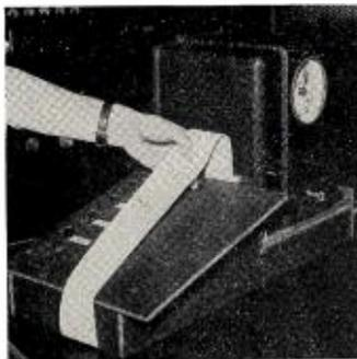
LOGGING CLOCK to record the station's programs and the hour, minute, second and fraction of a second on which each starts and finishes resulted when Mr. Pribble and S. E. Leonard, engineer in charge, got their heads together. Instrument provides foolproof check on what was aired and when.
