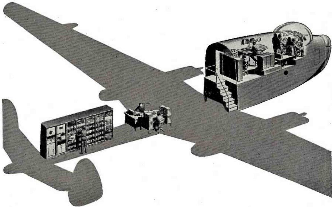
This is a "flight trainer"—an electronically operated replica of the PBM-3 flying boat. It was conceived by the Bureau of Aeronautics and developed by Bell Telephone Laboratories to train Navy bomber crews on the ground.
