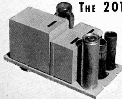
The 201 Series consists of the 201-A which has a single filter stage and 201-B which has a dual filter stage. The latter type is designed to supply filament and plate power for pre-amplifiers, such as Types 106 and 111. The 201 Series also supplies power for associated line amplifiers such as the Langevin 102 Series. Both units of the 201 Series possess excellent regulation and low ripple content.
