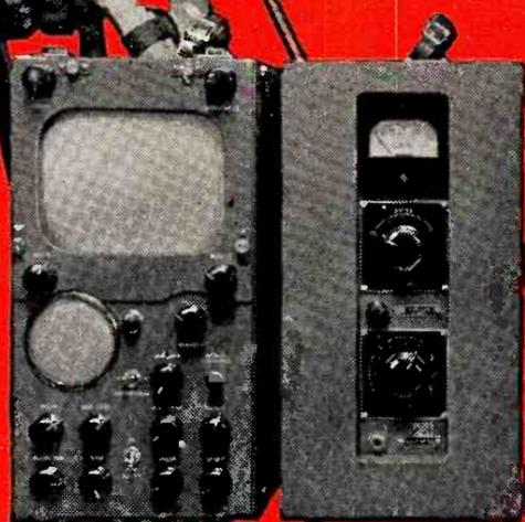
Duplicate camera control used for two-camera operation
