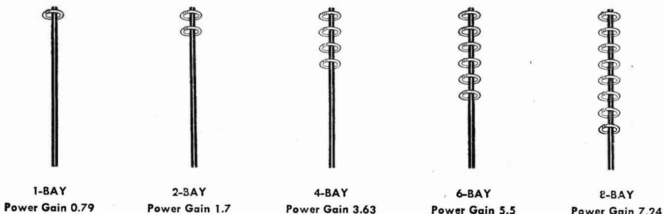
\*Compared with a standard half-wave dipole
