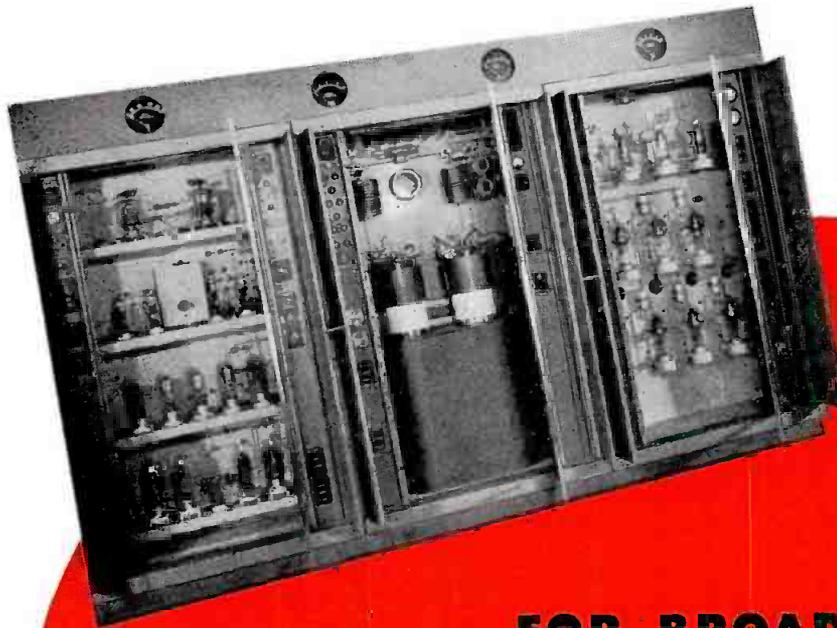
The CONTINENTAL Type 315 Transmitter, at left, offers a deluxe design for 5 KW AM operation. It has many features not ordinarily incorporated in transmitters of this class, including special equipment for matching transmitter output into sharply tuned loads often encountered in directional arrays.
