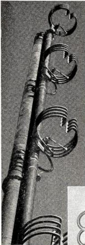
Above. Four sections of a BFA FM Antenna pole-mounted and interconnected by  $3\frac{1}{8}$ " coaxial transmission line.
