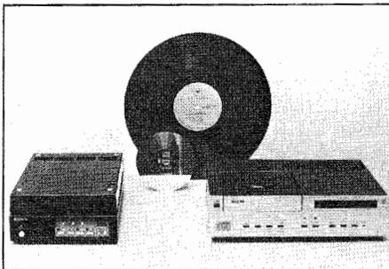
**Future disk.** Sony and North American Philips unveiled its new Compact Disc Digital Audio System in New York last week, announcing the 4.7 inch disk will debut in the fall of 1982. Proponents claim the digital record will make present recording obsolete, by eliminating distortion and prevent deterioration that occurs with current mechanical stylus systems. The disk contains an hour of playing time.
