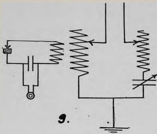
try constant changes of his inductance and capacity and compare the readings of his hot wire meter in the aerial leads with the distinctness in which surrounding stations are able to receive him. If this is done in a systematic manner, each receiving station making a record of the clearness, and condition of spark,
