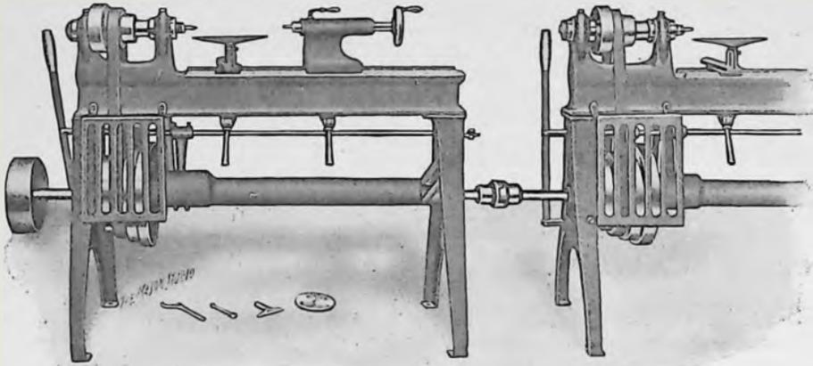
Have Silent Friction Clutch to start and stop each lathe separately. The lever for operating clutch automatically applies a brake to stop spindle. This NEW LATHE is made with 5 different methods of drive countershaft, underdrive, overhead friction drive, two styles of motor drive. Made with bronze boxes, ring oilers, 12 in. swing, and a variety of different equipments. Send for NEW MANUAL TRAINING CATALOG showing these and other machines for manual training work.
