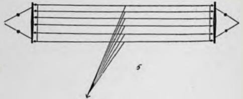
in clay is usually inefficient, and sand, unless wet, has a very high resistance. A station in the woods will lose much of its transmitting energy, if the aerial is near any trees. For this reason, when it is necessary to guy the antenna to trees, strain insulators should be cut into the guy wire at equidistant intervals to reduce this leakage factor.
