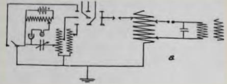
Condensers should have about from .001 to .005 M.F. capacity. The potentiometers should be at least 300 ohms resistance, when two or more cells of battery are used.
