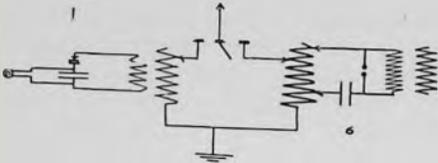
the antenna depend entirely upon the capacity of the station. When a brush discharge is observed from the aerial, it is generally a safe sign that more aerial wire is required.
