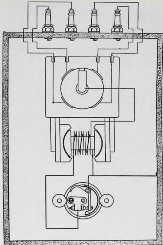
Fig. 14.—Wiring diagram of Type "C" systems (with external transformer).
