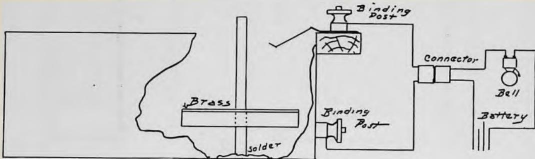
The float is constructed of cork or wood, having a diameter of 3 in. Over this is tacked a piece of  $\frac{1}{32}$  in. sheet brass. Through their centers a sleeve having  $\frac{1}{4}$  in. inside diameter is placed, using care that both sleeve and brass make good contact. The contact spring is made of a piece of spring brass,  $\frac{1}{32}$  in. thick, bent into the form shown in the drawing. The spring is connected by
