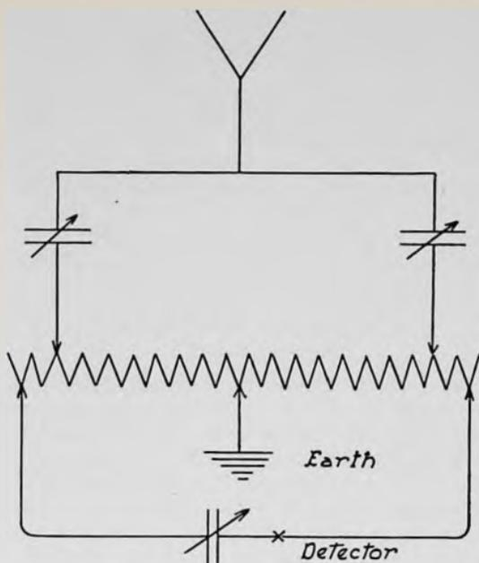
best tuned to the received impulses. If these impulses consist of a sufficiently long train of waves, discrimination is effected between these and any other impulses (even if of the same periodicity), if such other impulses are of a more rapidly damped character. A "valve receiver" interference preventer based on a similar principle has been patented by Marconi.
