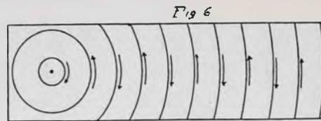
As we saw from Experiment 1, that when we pass an alternating current along a wire, we get an alternating magnetism, we shall expect to get an alternating magnetism in this case, and, in fact, we do. The current forms circular rings of magnetism around the wire just as in Experiment 1, the rings being piled on top of each other from the ground up to the top of the wire in the form of a big cylinder.
