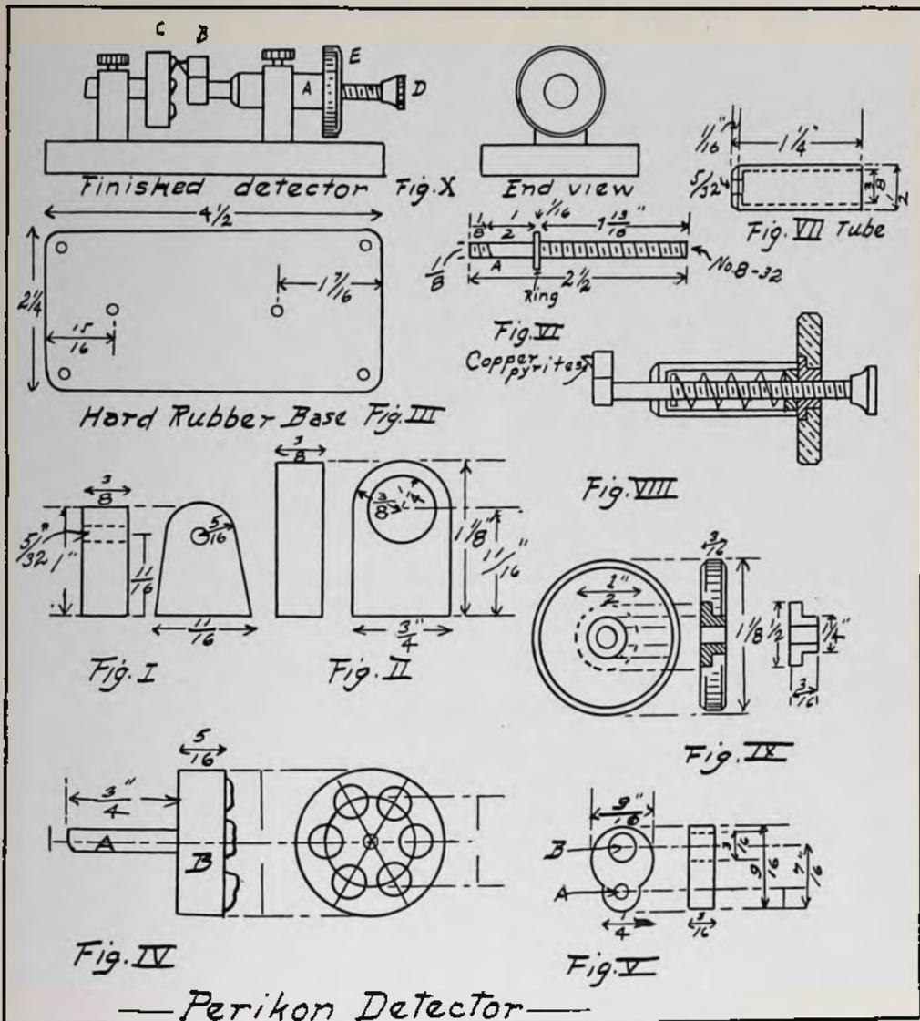
pyrites' holder is shown in Fig. 5, and is best made by following closely after the figure. The hole A is threaded, and B is not drilled quite through.
