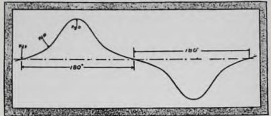
Fig. 12.—Electrical pressure fluctuations and changes in direction of flow in the armature winding through one complete revolution.
