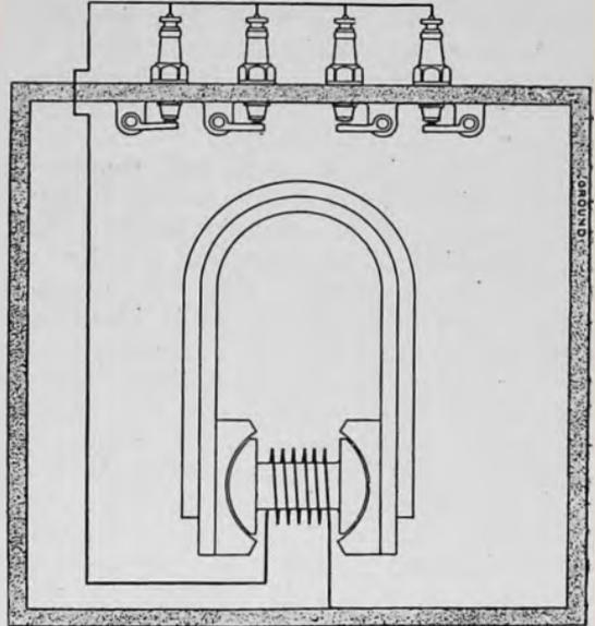
Fig. 13.—Wiring diagram of Type "A" (Make and Break) Systems.
