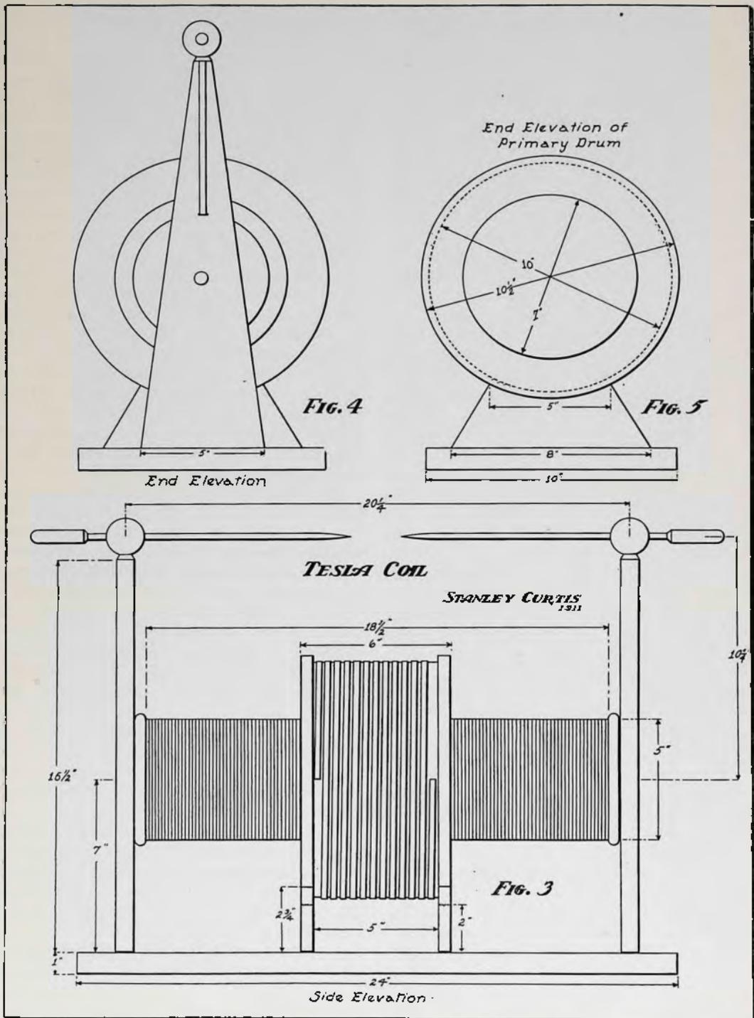
be spaced about the width of a piece of the wire apart. There are several methods of doing this, and the easiest and best is to use the screw-cutting lathe with the gears set to cut a No. 56
