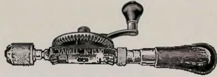
The "Yankee" Hand Drill, No. 1530, has a right and left-hand ratchet movement, and is made on lines similar to the regular "Yankee" Breast and Hand Drills. The size, however, is somewhat smaller, and the tool is intended for light work. By moving the small shifter on cylinder between small gears on the spindle, the various combinations of the ratchet and gears are brought into play.
