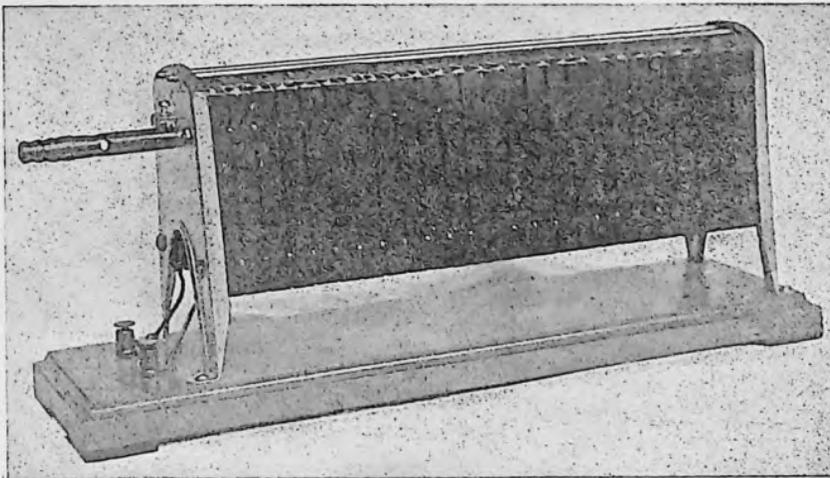
directly through the apparatus between the copper tubes, the round tube being perforated at intervals throughout its entire length, the ends of the series of elements of this thermo-generator are connected to terminals supplying the current to a storage battery of two to four volts, for charging the same or for illuminating small surgical lamps or operating faradic coils.
