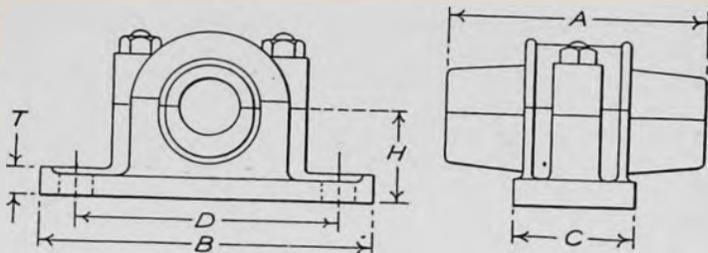
Fig. 14. Ring-oiling Ball and Socket Pillow Block
