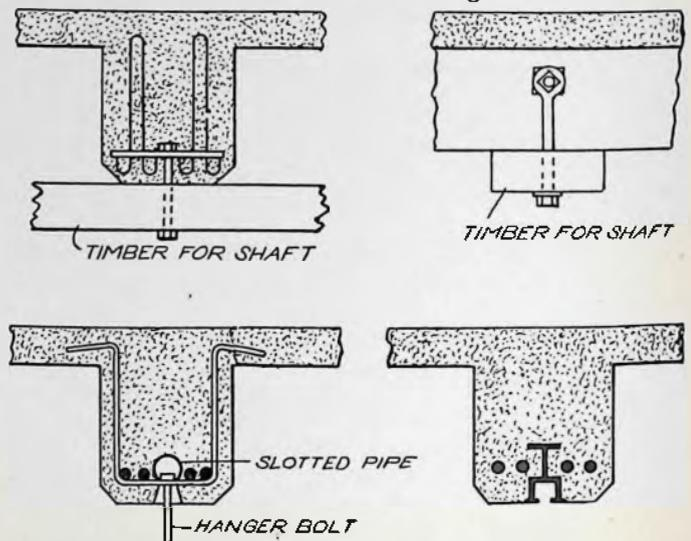
Fig. 13. Methods of Supporting Shaft Hangers on Reinforced Concrete
