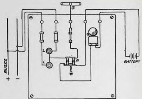
CONNECTION FOR ALARM GROUND DETECTOR
