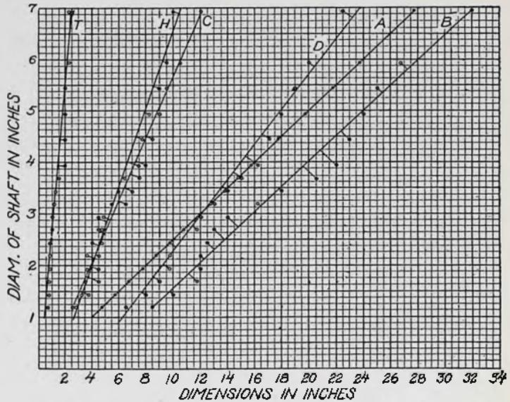
Fig. 15. Proportions of Ring-oiling Ball and Socket Pillow Block
