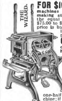
FOR \$16.95 we furnish one of the best concrete block machines and outfits ever made for making standard 8x8x16-inch blocks, the equal of machines others sell at \$75.00 to \$125.00. Our marvelously low price is based on cost of material and labor, with just our one small percentage of profit added.
