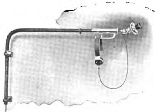
TRANSMITTER ARM WITH HEAD TELEPHONE.
