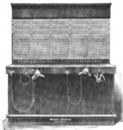
MAGNETO MULTIPLE SWITCHBOARD
