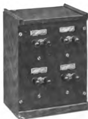
ALARM FOR TELEPHONE SYSTEMS.
