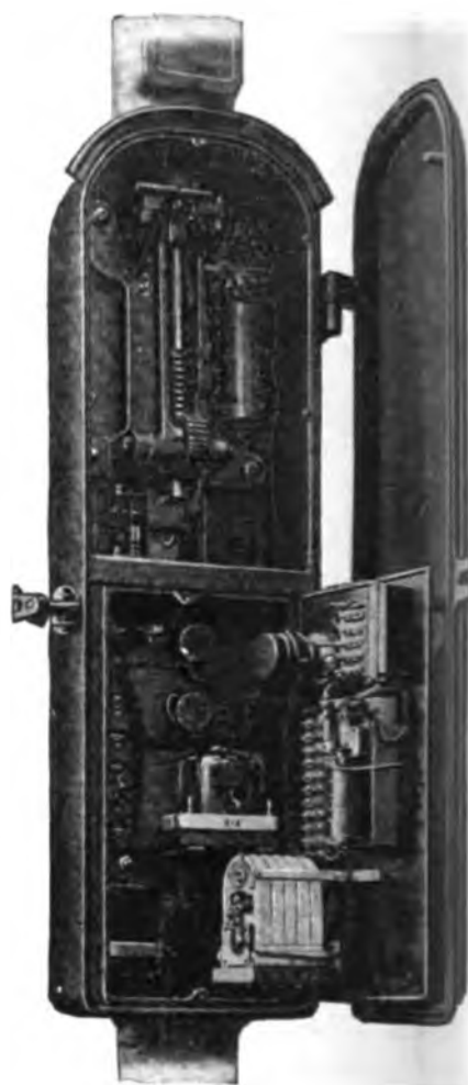
FIG. 2.—SIGNAL AND TELEPHONE APPARATUS IN BOX.
