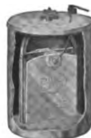
Size over all, 7 1/2 x 11. Jar only. Inside dimension, 6 1/2 x 8 1/2. Edison- BSCO Type 403 Cell 400 A. H. Capacity, furnished with either porcelain or heat resisting glass jar.
