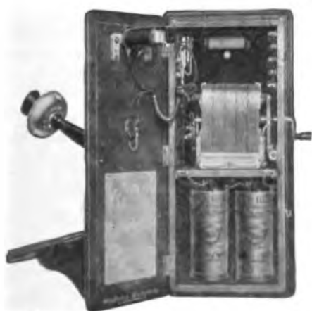
FIG. 1A—MAGNETO WALL SET—OPEN.
