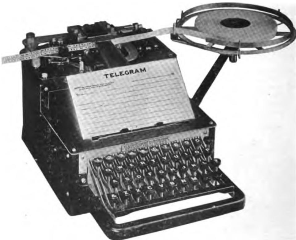
FIG. 2—FRONT VIEW OF PERFORATOR.
