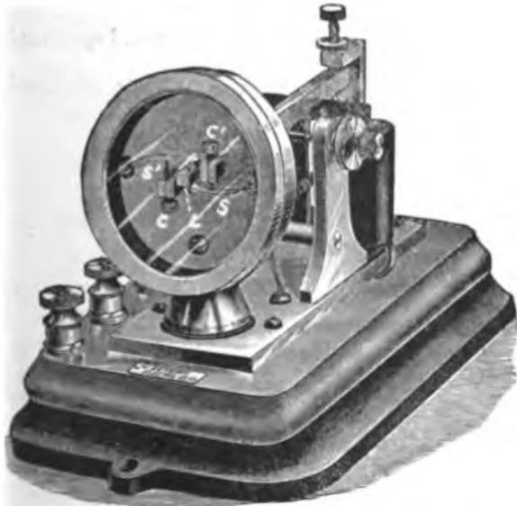
FIG. 66—ONE FORM OF POLE-CHANGING INSTRUMENT.
