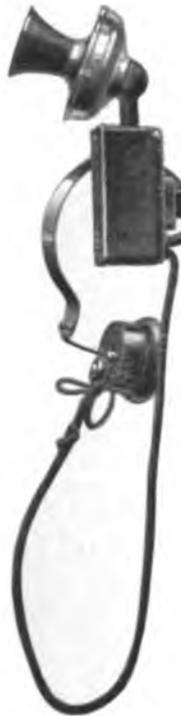
is made to meet the severe requirements of railroad work. It is arranged for both wall and desk mounting. The arm is the complete telephone set; all coils, condensers and terminals are located in the base and readily accessible for inspection. The transmitter key is located in a convenient place in the
