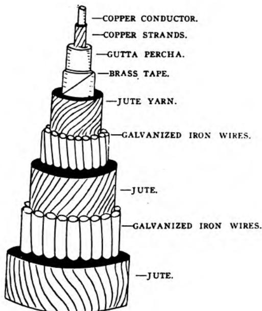
SHORE END TYPE OF CABLE WITH VARIOUS LAYERS STRIPPED.
