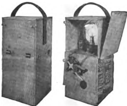
FIG. 2—PORTABLE SIGNAL OUTFIT WITH TELEGRAPH KEY.
