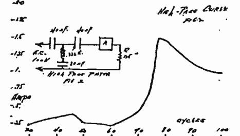
In Figure number two the curve is self explanatory. It starts at .25 of an ampere, increases slightly only to decrease to a minimum value of .20 at 60 cycles. It increases then to a maximum point of 1.5 amperes at 76 cycles. From this position it decreases gradually to 100 cycles where the current is little less than one ampere. The entire condition may be classed as one of high current at high frequency and low current at low frequency.
