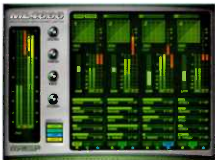
McDSP ML4000 multiband processor applies different dynamic processing to different frequency ranges in a mix.
