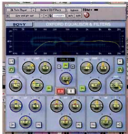
This Sony Oxford EQ is being used to roll off the low and high extremes. This creates headroom in the mix while maintaining the track’s sound.
