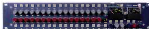
A summing mixer like this Neve 8816 can add analog warmth to a digital mix.
