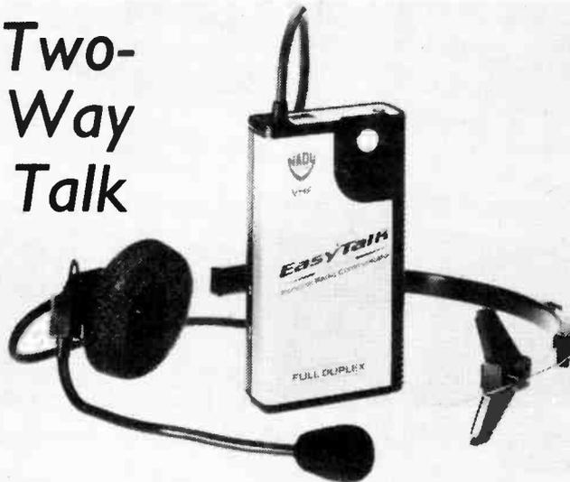
The newest addition to Nady Systems' "Easy Talk" personal radio communicators is the PRC-3, a receiver/transmitter equipped with headset and body pack complemented by a belt clip, adjustable microphone boom, head-phone volume control, stowable whip antenna, and an optional extended battery pack. Operated at the 49 mHz FM band via a nine-volt battery, the unit can be used in both play and work situations. For more details regarding price and availability, contact Steve Caraway at (415) 652-7632.
