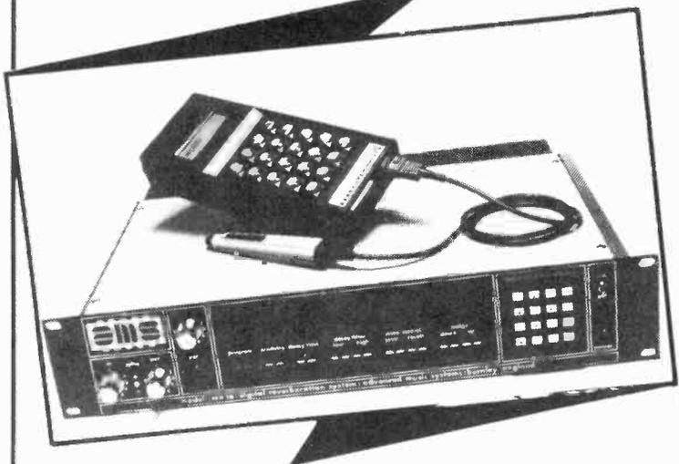
**Advanced Music Systems** has designed the RMX 16 digital reverberation unit, whose nine programs encompass small room and concert hall simulations plus echo and special effects. It features an 18 kHz bandwidth and 90 dBA dynamic range. A remote terminal is also available with bar code reader input.
