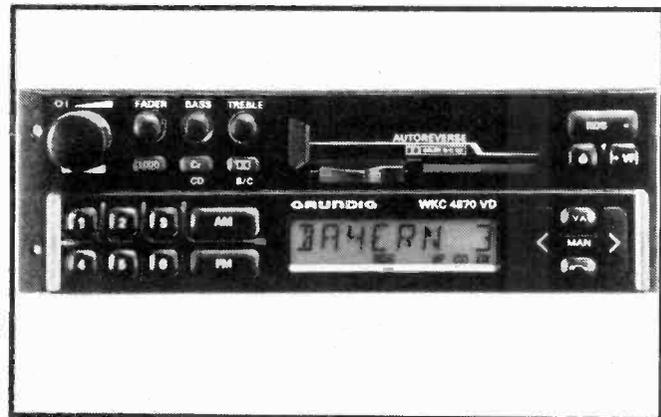
Grundig RDS-equipped receiver displaying West German Bayern 3 network station
