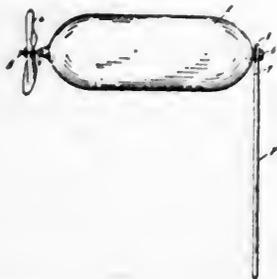
In a toy balloon construction, the combination with a bladder having an inflating neck and a handle in the form of a rod provided with a slot at one end thereof which is adapted to receive said inflating neck in twisted or folded condition and retain the same, thereby to prevent the escape of the gas within the bladder, said rod extending at substantially right angles to the axis of the bladder.
