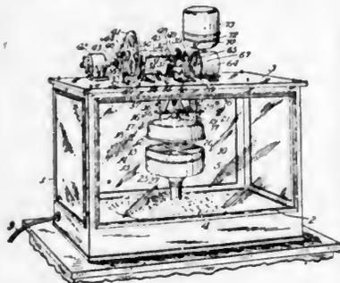
A corn-popping machine having a stationary concave pan, a heater arranged below the pan, a rotary shaft guided above the pan, a pan cover movably guided on the shaft, and a hub secured to the shaft and having agitator fingers thereon extending from the lower portion upwardly across the surface of the pan.
