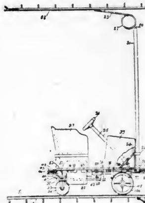
In an amusement device, a contact floor, a contact roof, a vehicle adapted to move on said floor and have a portion in contact with said roof, a motor mounted on said vehicle deriving its source of current thru the contact of said roof and said floor contact, and a portion of said floor adapted to move to impart movement to the vehicle independent of its own motive power.
