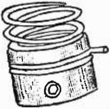
**TURNTABLE CLUTCH ASSEMBLY FOR ALL MODEL WURLITZERS**
