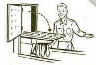
Loosen 2 clips to swing open the picture frame moulding of litebox - then entire insert with reels and wiring folds forward
