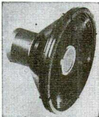
The following are the manufacturer's specifications and performance claims; nominal response is 30 to 15,000 cps, power rating is 30 watts (U. S.), impedance at 400 cps is 15 ohms, bass resonance is 40-45 cps and cross-over frequency is 2,000 cps. The speaker is available in the U. S. thru Ercona Corporation, N. Y. C.
