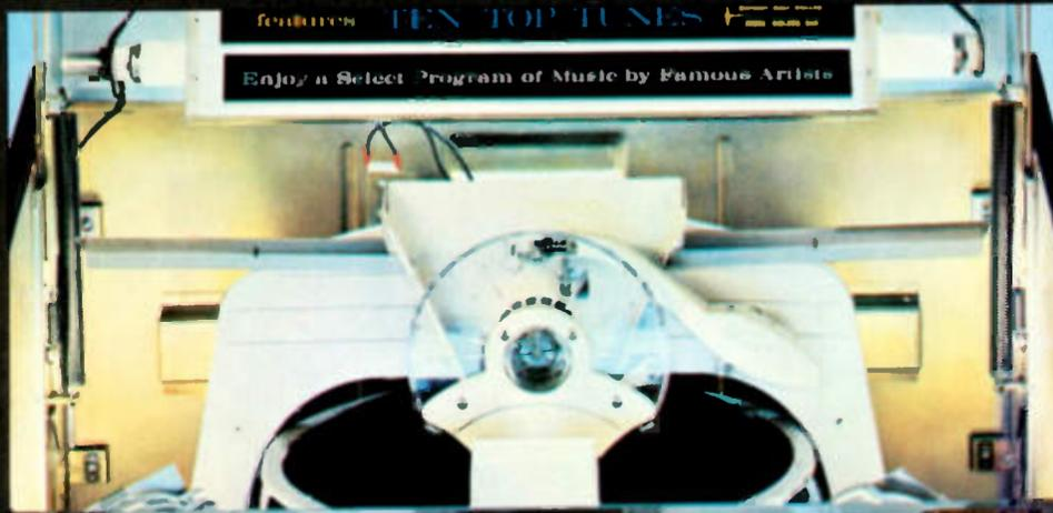
**NEW SPRING-LOADED DOME** — Unlock the dome and it lifts automatically to finger hold clearance. Raise to latch position with almost effortless action. It can't drop even if a spring should fail. As dome is opened, the title strip holder can be dropped into loaded position and is held firmly in place while strips are changed. Programming, record changing, needle replacement and tone arm adjustments are all quickly performed. Dome closes with the same hydraulic-like cushion action.
