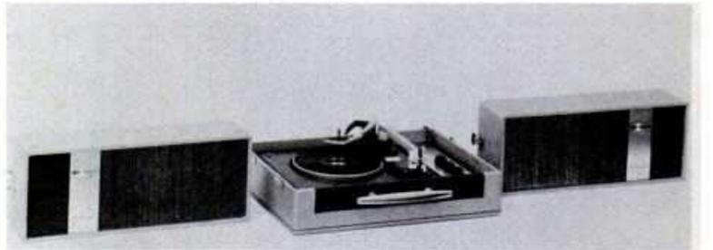
Automatic stereo phonograph by Capitol. Dual-channel six-transistor amplifier, 10-watt power, frequency response 50-12,000 cps. Two six-inch ceramic magnet speakers in separate enclosures, Garrard four-speed automatic changer. Turnover cartridge, three controls. List price \$99.95.
