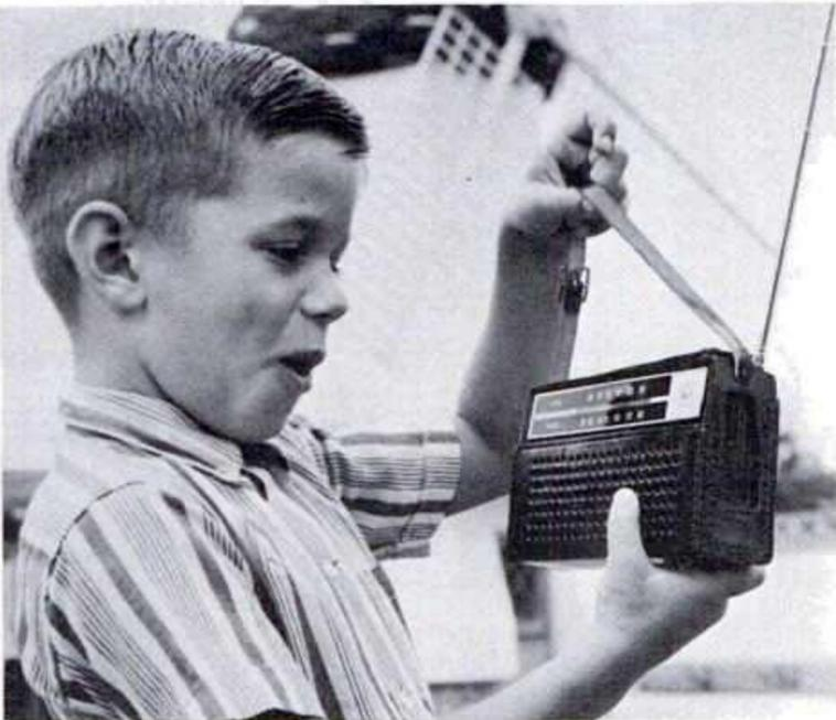
RCA'S NINE-TRANSISTOR portable radio features FM-AM reception, telescoping FM antenna and built-in AM antenna. Equipped with slide-rule vernier tuning, personal earphone and carrying case. Price \$27.95.
