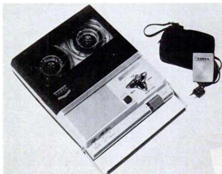
**SOLID-STATE VISTA** tape recorder by Craig Panorama. Two-speed, "T" function controls for play, record and fast forward, automatic level control. Frequency response 150 to 7,000 CPS at 3 3/4 speed, 200 ohm remote-control microphone, operates on six "C" batteries. Price \$39.95, includes earphone and accessory pouch.
