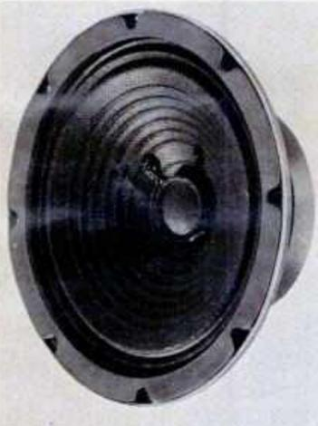
A THIN PROFILE coupled with a large magnet are the exceptional features of Utah Electronics new C5FC stereo speaker for car doors. The new speaker is five inches in diameter, boasts a 5.5 ounce barium ferrite magnet but has a depth of less than two inches. It will handle 10 watts of program material and a moisture resistant cone prolongs speaker life.
