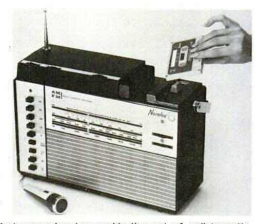
Most comprehensive combination yet of radio-cassette equipment in this multi-band portable. Recording is possible direct from radio to cassette.
