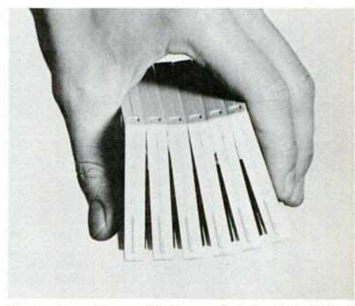
Six musicassettes, each the equivalent of an LP at present and ultimately a double LP, fit into the hand. Four present-day cassettes offer up to 240 minutes playing time compared with the 80 minutes of a cartridge which occupies the same space, Philips claims.
