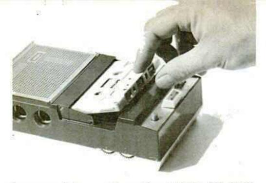
Forerunner of the cassette equipment, Philips' EL 3300 battery-operated tape recorder. Later versions, the 3301 and 3302 incorporated design modifications but are physically identical.
