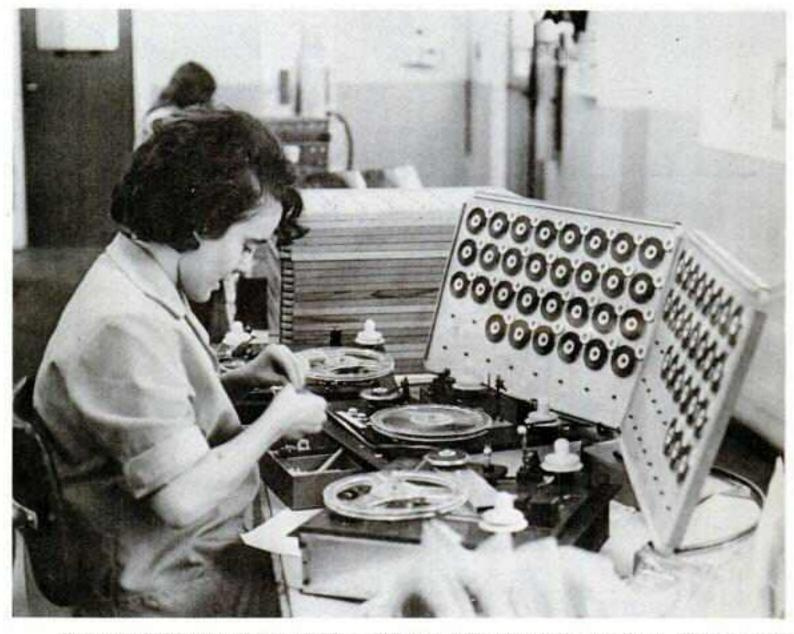
Spooling the virgin tapes for the C60 and C90 Compact cassettes. Three spools of blank tape are handled at a time: one has leader tape and hub spliced on; another spools tape onto the hub; and the third has trailer tape and hub secured.
