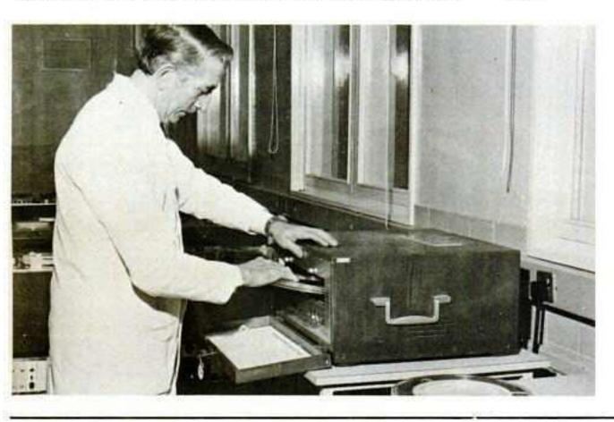
Dubbing operator Harry Munson bulk erases a spool prior to a dubbing run-through. Each spool of tape is erased using the Weircliffe bulk eraser to ensure absolute conformity of magnetic influence prior to the duplicating procedure.
