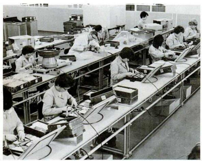
A general view of part of the cassette assembly section. Each operator is trained to perform various assembly procedures to relieve boredom and also provide facilities for concentrating on specific tasks if a rush develops.
