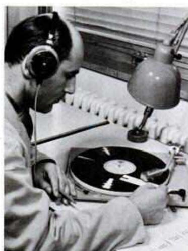
When a defect is recorded, the slip of paper is transferred to the disk to indicate the exact place on the record where the fault is to be found.
