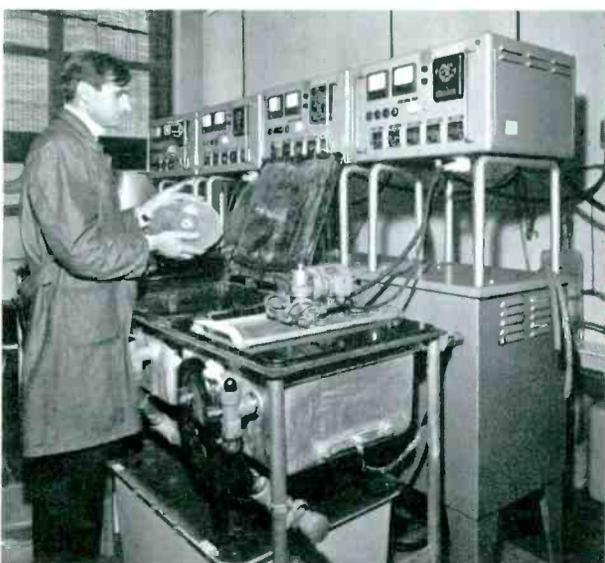
*The electro plating system used for the production of metal parts to press records.*
